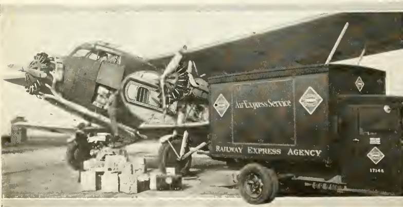
Loading air express packages aboard a trimotored Boeing of United Air Lines
